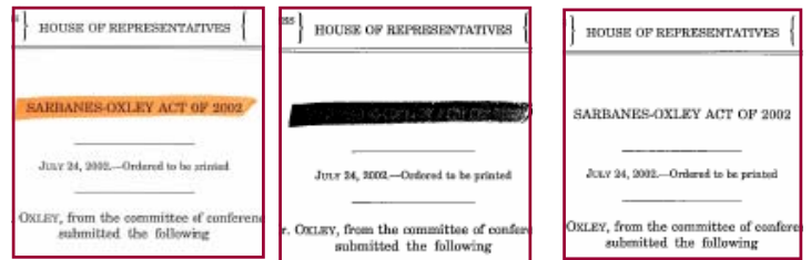
Left: This is an original document with highlighting. Middle: Original scanned in Monochrome mode results in highlighted areas being unreadable. Right: Original scanned with color dropout renders the document instantly usable with no human intervention required
